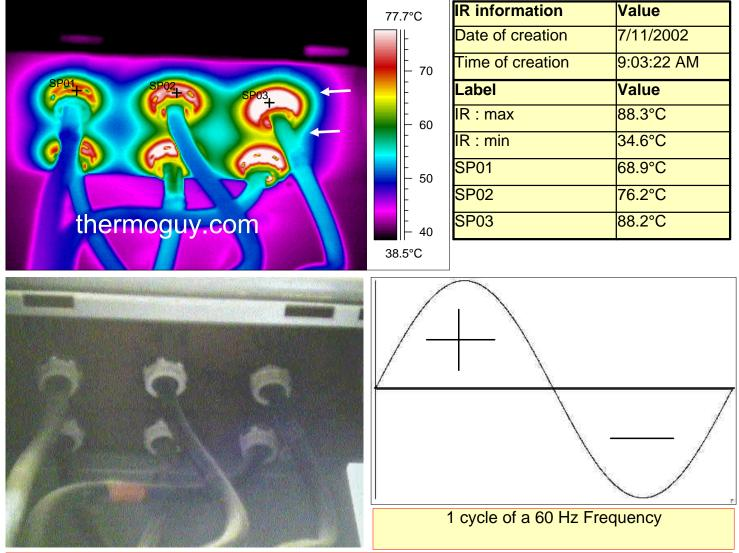
Example of Extremely Low Frequency (60 Hz) Causing Electrical Failure
